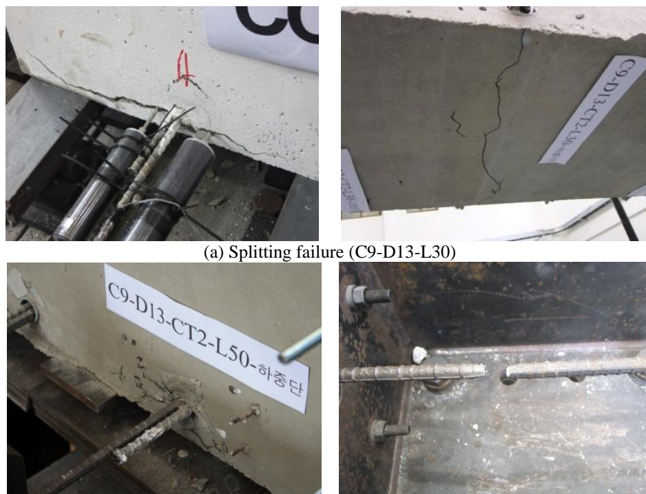
(b) Tensile failure of bar (C9-D13-L50)
